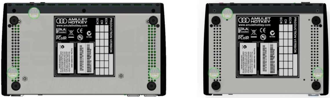
Figure 1: Position of tamper seals on zero clients
