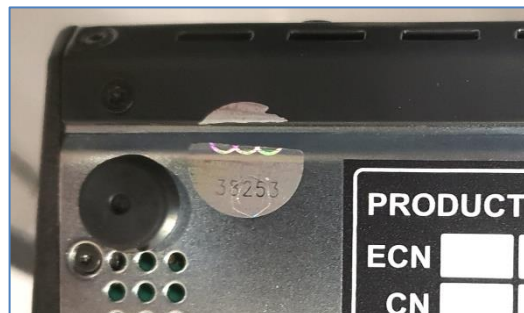
Figure 2: Example of a faulty anti-tamper seal
